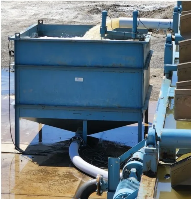
The system separates the suspended solids and brings them out in a thickened form that does not require secondary processing.
